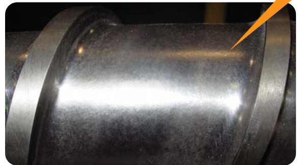
▲ Typical poor adhesion and chipping of competitive carbide coatings Xaloy's X8000™ has a metallurgical bond exhibiting no chipping ▼
